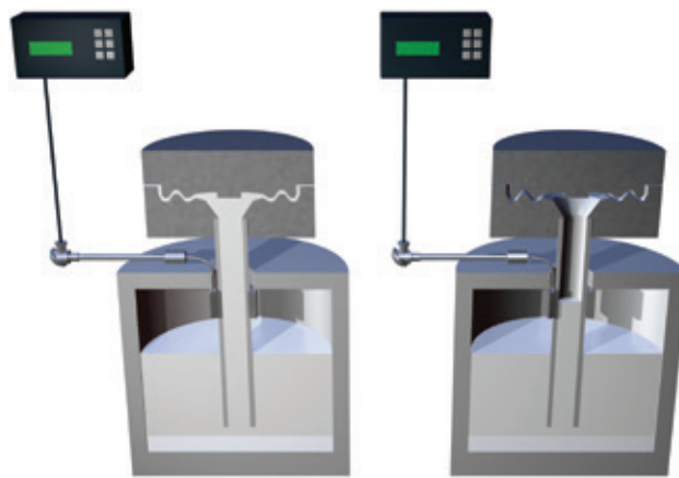
RP used to control the metal level in a riser tube.
